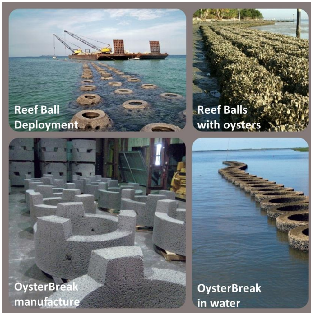
Figure 6. Precast Concrete Designs
