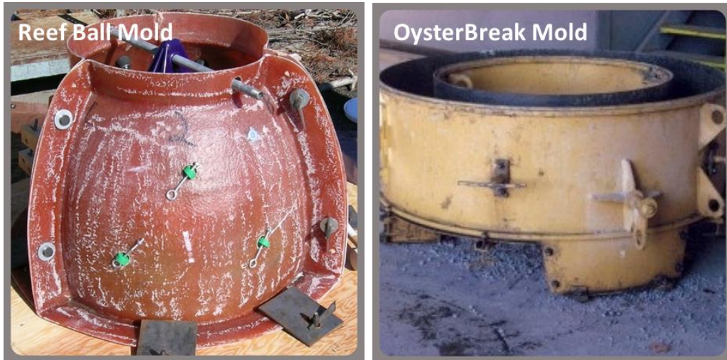
Figure 10. Precast Concrete Molds
