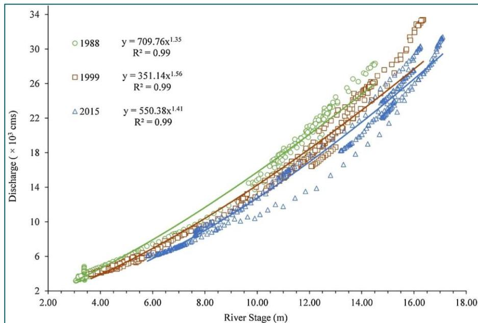
Figure 3.19: Example of Stage-Discharge rating curve (Wang and Xu 2016).
