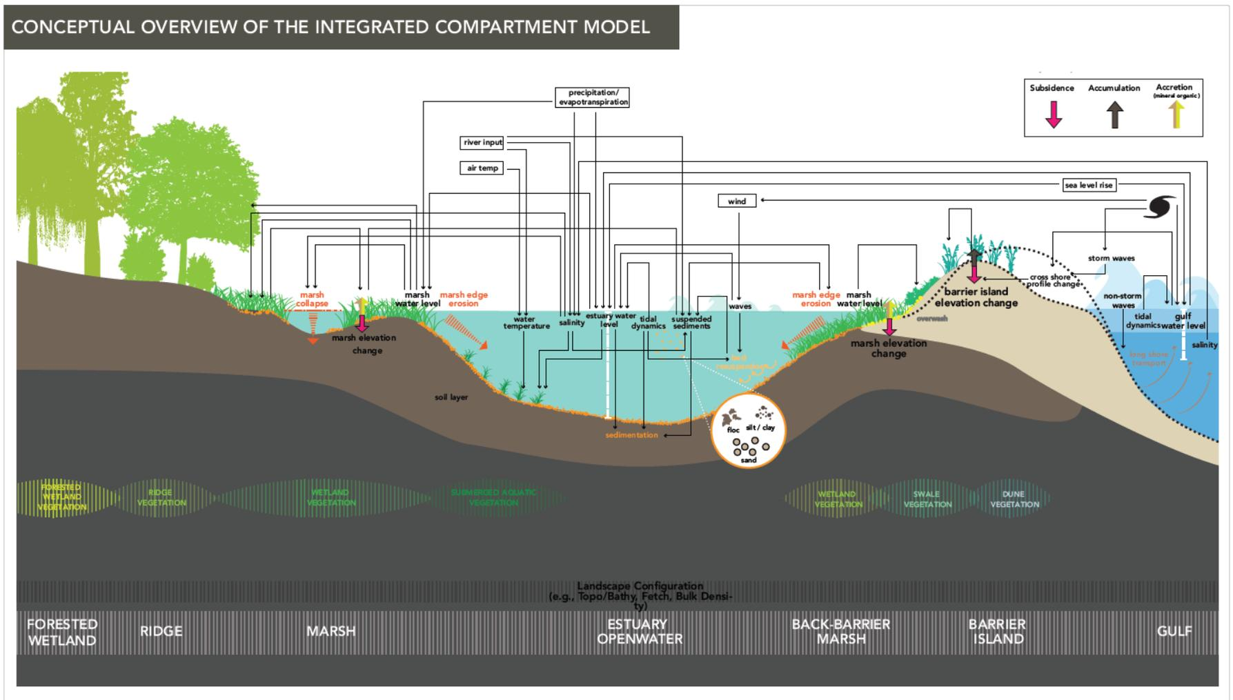
Figure 3.18: Major physical processes and linkages contributing to MRD simulations conducted as part of the 2017 Coastal Master Plan (Figure 3.5, CPRA 2017).
