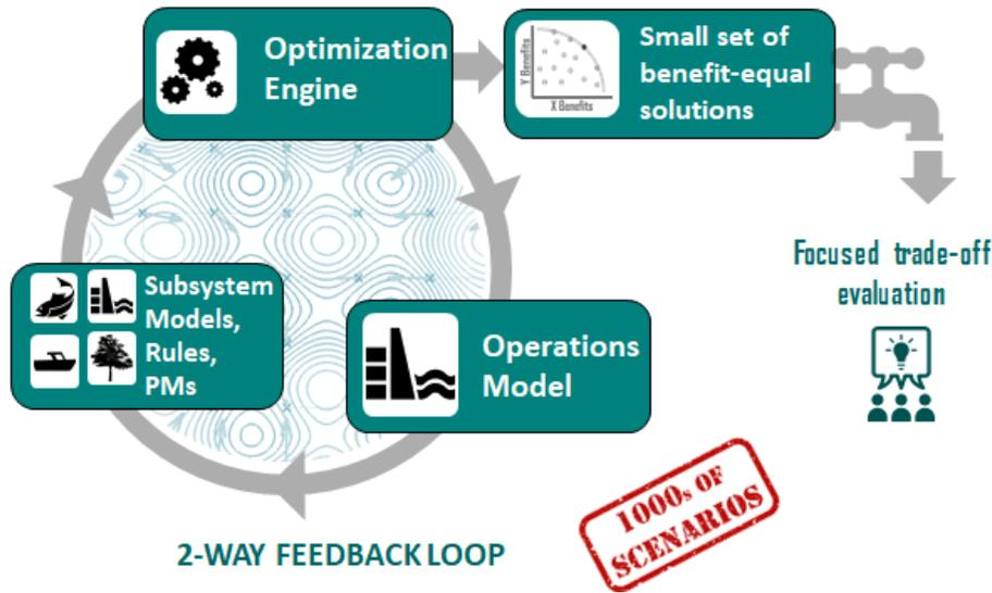
Figure 1.5: Example of an advanced tool feature, termed Turn-Taking Optimization. Illustration represents coupled decision support models and performance measures functioning within a two-way feedback loop and linked to optimization algorithms that help narrow down best candidate solutions for decision-makers.
