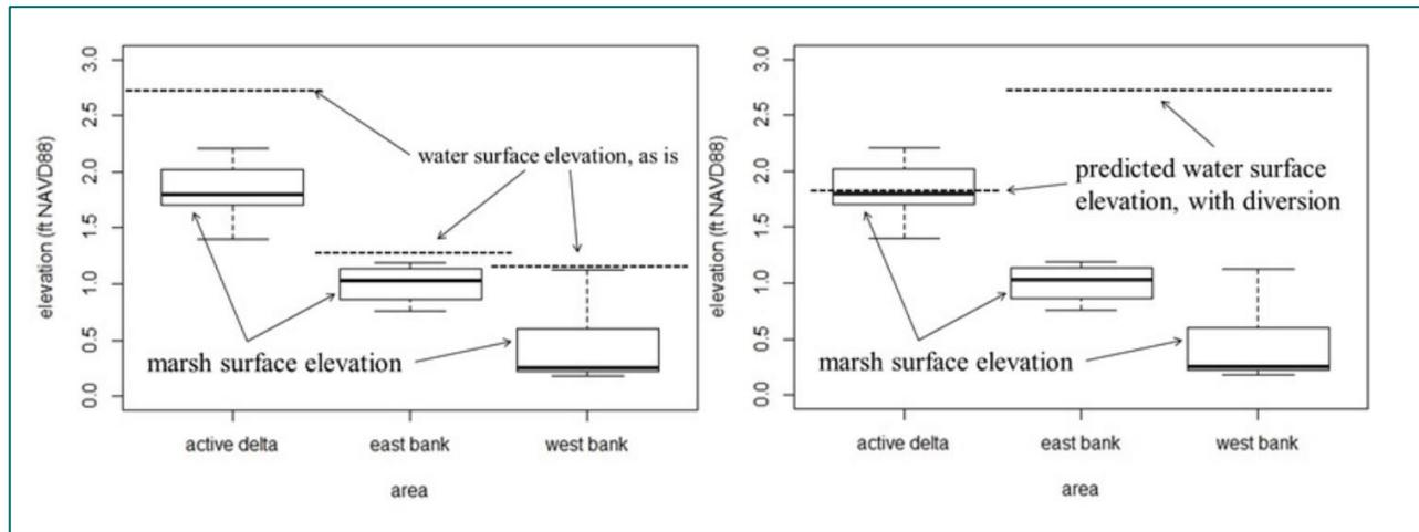
Figure 3.3: Example of hypothetical changes in water elevation with (right) and without (left) multiple diversions in operation on both sides of the river. In this hypothetical example, surface elevation in Barataria Bay (west bank) increases by about 2 feet when the diversions are active (Peyronnin et al. 2016).
