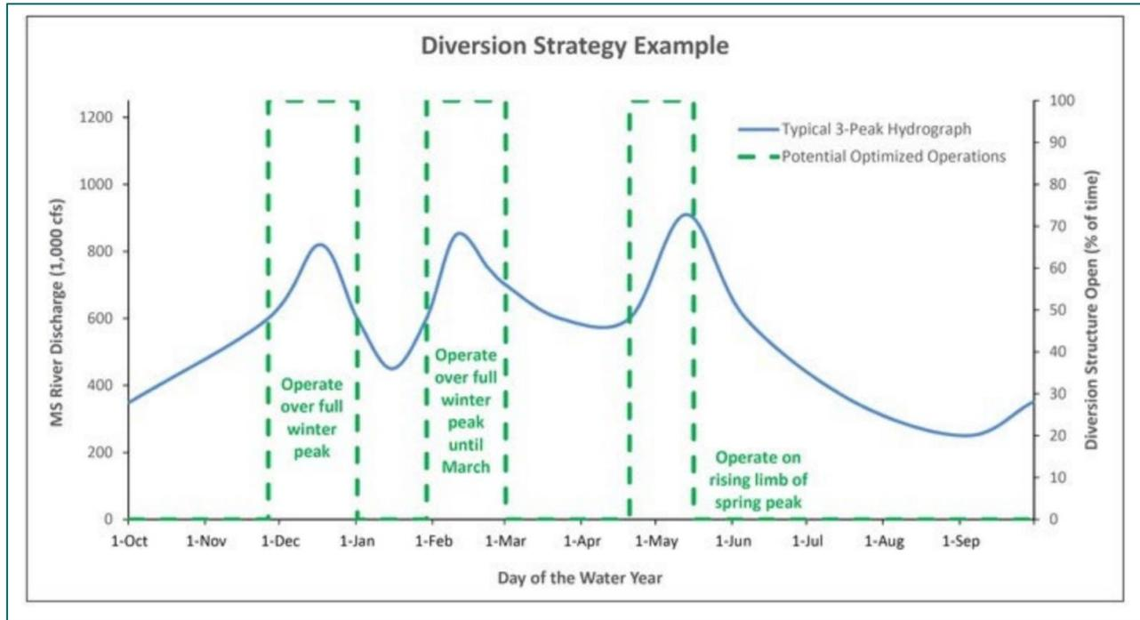
Figure 1.4: Simplified conceptual example of how a diversion could be operated to deliver sediment in consideration of its effects on fish and wildlife habitats. As noted in Peyronnin et al. (2017), an operation strategy can be developed and tested for each hydrograph typology (demonstrated here on a three-peak hydrograph typology) that effectively captures sediment for land building, while also balancing the needs of the ecosystem and communities.
