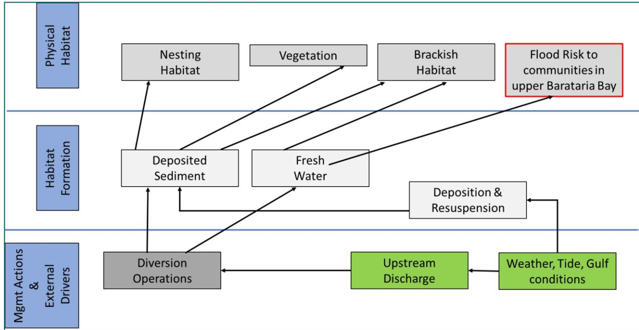
Figure 3.4: Simple representation of the conceptual relationship between the input of fresh water at the diversion potentially leading to flooding of communities in upper Barataria Bay.
