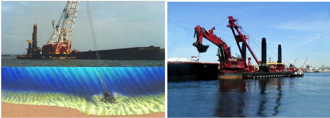
Figure 4. Mechanical dredges: crane (left) and excavator (right)
