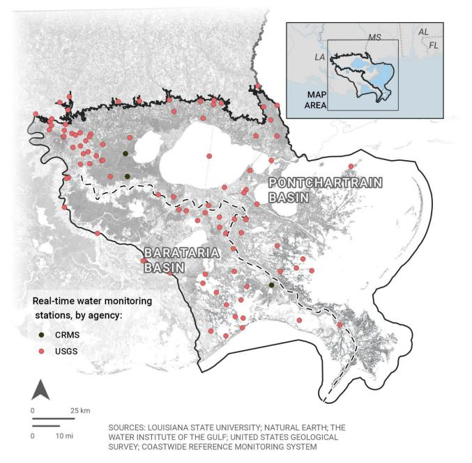
Figure 2.5: Locations in the lower Mississippi River, Barataria Basin, and Pontchartrain Basin with a subset of <u>real-time</u> monitoring by U.S. Geological Survey (USGS) broadly (red dots) and specifically within the Coastwide Reference Monitoring System (CRMS) (black dots).
