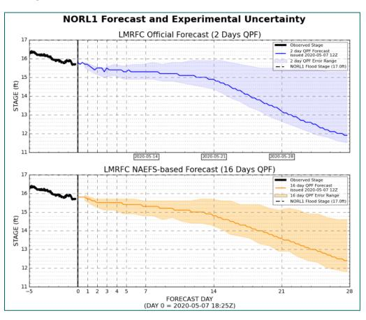
Figure 3.20: Example of NWS 2- and 16-day stage forecasts at New Orleans provided through the AHPS.
