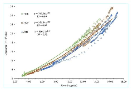
Figure 3.19: Example of Stage-Discharge rating curve (Wang and Xu 2016).
