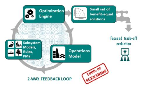
Figure 1.5: Example of an advanced tool feature, termed Turn-Taking Optimization. Illustration represents coupled decision support models and performance measures functioning within a two-way feedback loop and linked to optimization algorithms that help narrow down best candidate solutions for decision-makers.
