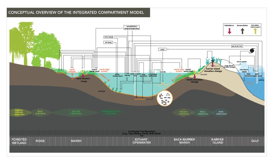
Figure 3.18: Major physical processes and linkages contributing to MRD simulations conducted as part of the 2017 Coastal Master Plan (Figure 3.5, CPRA 2017).
