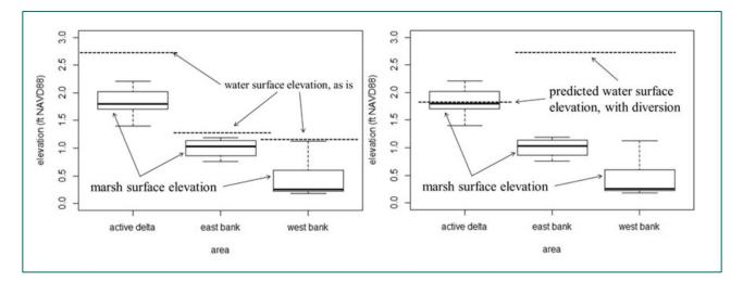
Figure 3.3: Example of <u>hypothetical</u> changes in water elevation with (right) and without (left) multiple diversions in operation on both sides of the river. In this hypothetical example, surface elevation in Barataria Bay (west bank) increases by about 2 feet when the diversions are active (Peyronnin et al. 2016).
