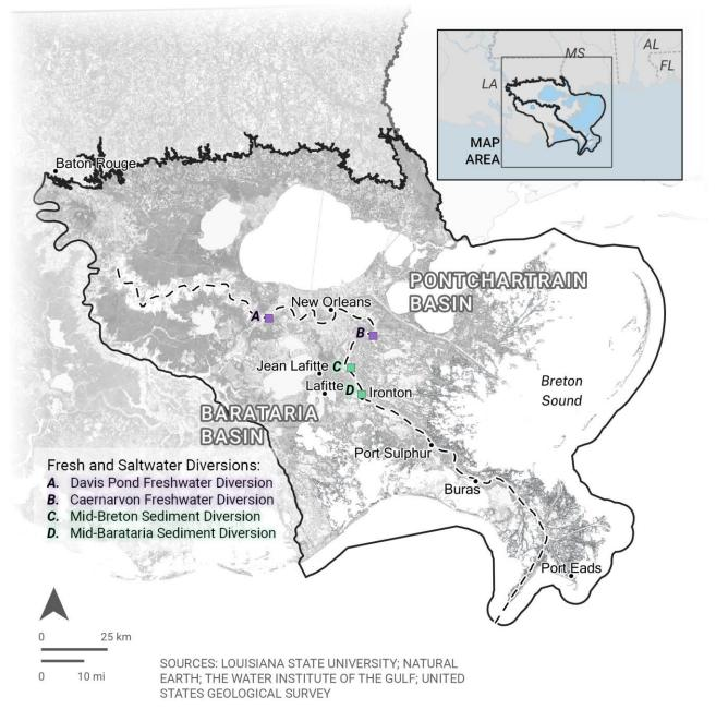
Figure 2.2: The two main basins and the discharge locations of planned (green) and existing (purple) freshwater and sediment diversion projects.
